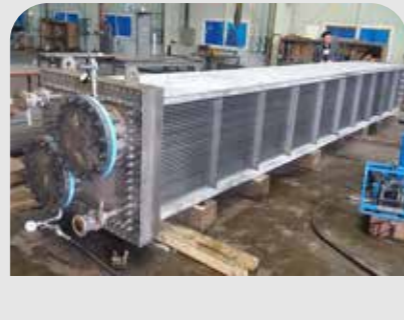
After Cooler Bundle
