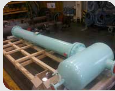
After Cooler Bundle & Separator
